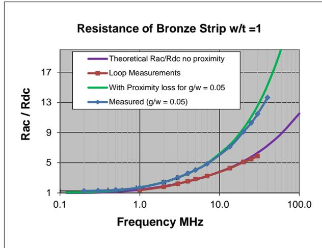
Figure 8.1 Comparison of equations with measurements
