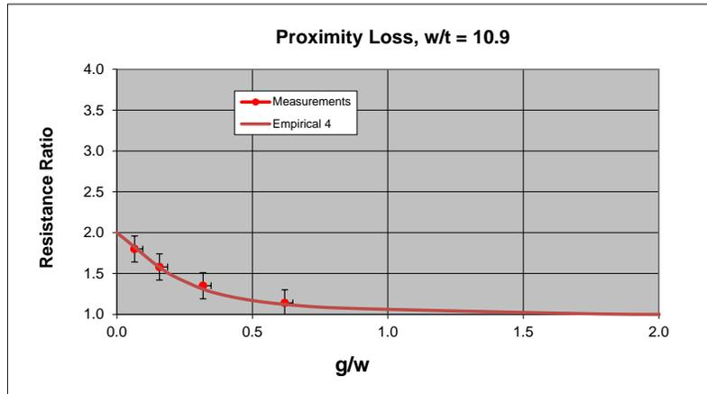
Figure 4.3.3 Limit of proximity loss for  $w/t = 10$
