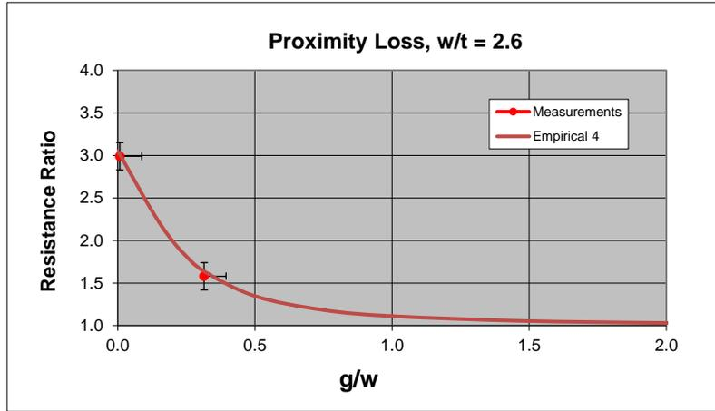
Figure 4.3.2 Limit of proximity loss for  $w/t = 2.6$
