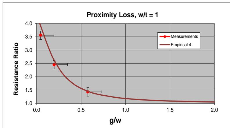
Figure 4.3.1 Limit of proximity loss for  $w/t = 1$
