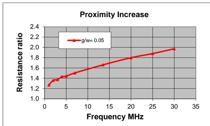
Figure 3.1 Increasing proximity loss with frequency
