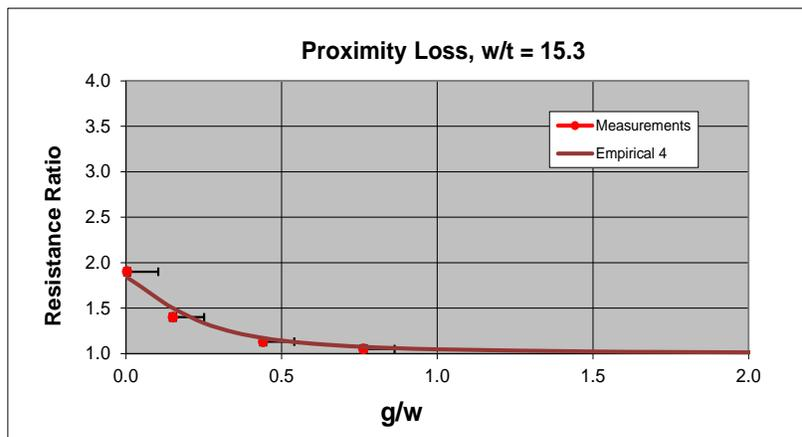
Figure 4.3.4 Limit of proximity loss for  $w/t = 15.3$
