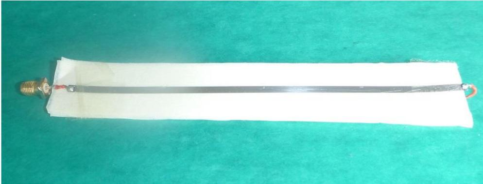
Figure A 1.1.1 Nichrome strips with spacer
