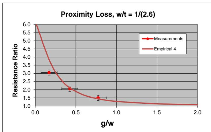
Figure 5.1 Limiting proximity loss Configuration 2,  $w/t=2.6$
