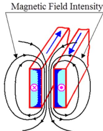
Figure 1.2 Magnetic field and current density in parallel conductors
