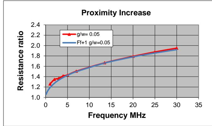
Figure 3.2 Measured proximity loss with  $(1+k F_{(f)})$
