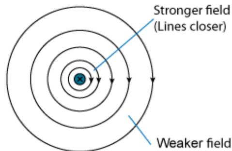
Figure 2.1.1 Lines of constant Magnetic Intensity  $H$  around a wire carrying a Current
