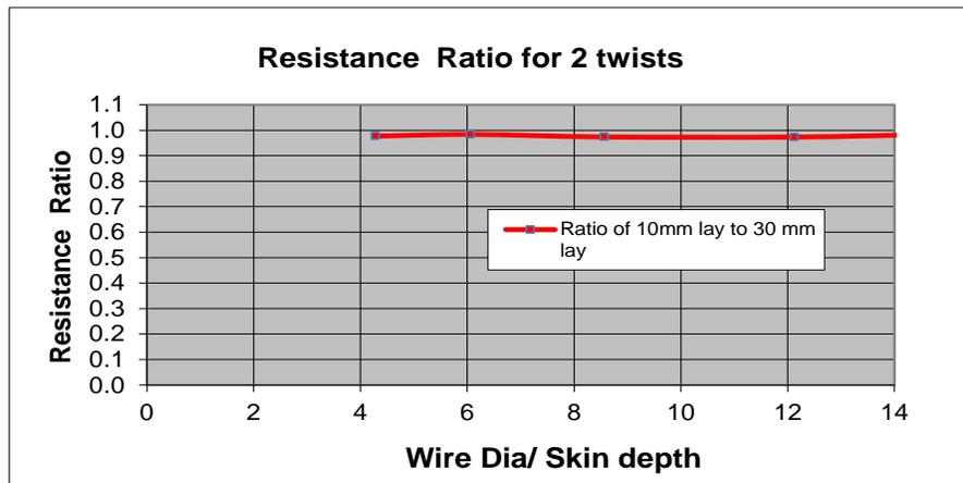
Figure A2.3.1 Measured Resistance Ratio for two Values of Twist
