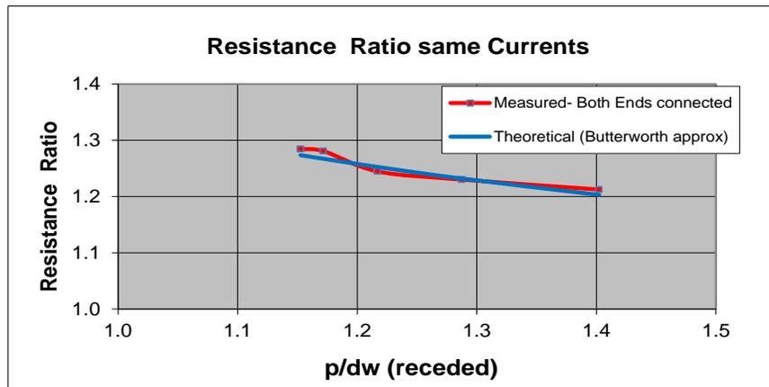
Figure A2.2.1 Resistance Ratio for Currents in Same Direction : Measured and Theoretical
