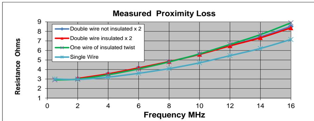
Figure 3.3.4.1 Measured Resistance: Currents in Same Direction
