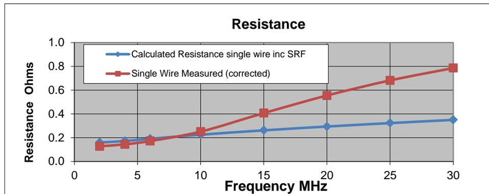
Figure A4.1 Resistance of Nichrome wire, Measured and Calculated
