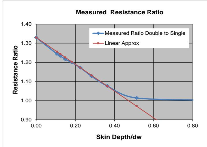
Figure 3.3.5.1 Measured proximity effect of two wires: currents in same direction
