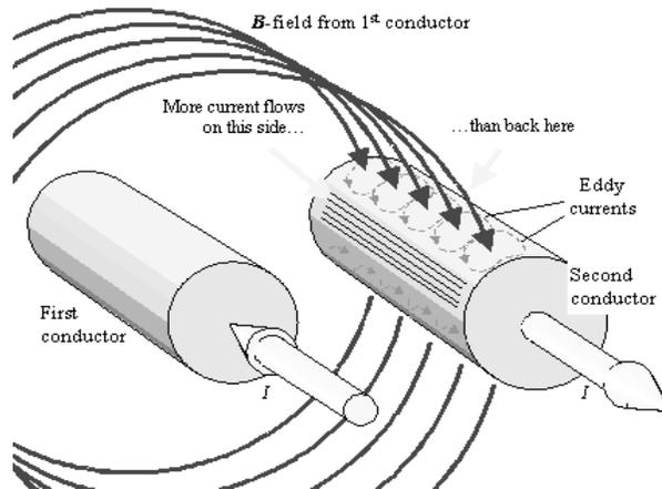
Figure A1.1 Induced Currents in Twin Wires
