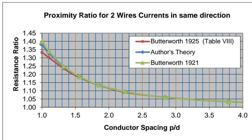
Figure 3.2.1 Theoretical Resistance Ratio for Currents in Same Direction
