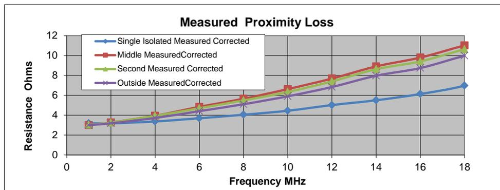
Figure A5.2.1 Resistance of Wires in a Group of Five
