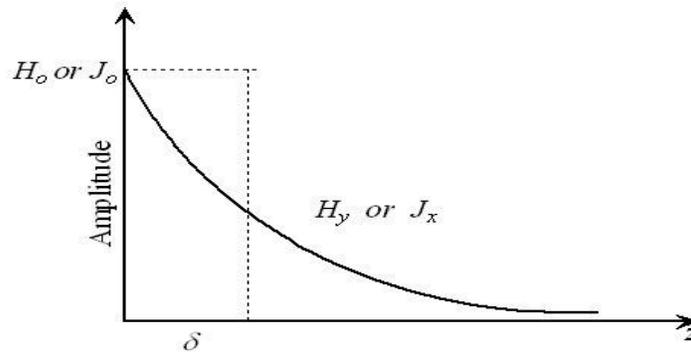
Figure 2.2.1 Current density at high frequencies
