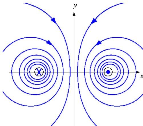
Figure 4.1.1 Lines of constant  $H$  around Two parallel Wires carrying Opposing Currents
