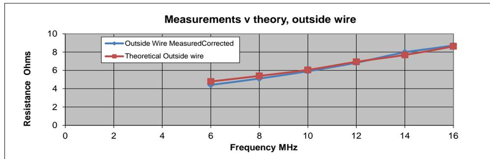
Figure A5.4.2 Resistance of Outside Wire of Five Wires
