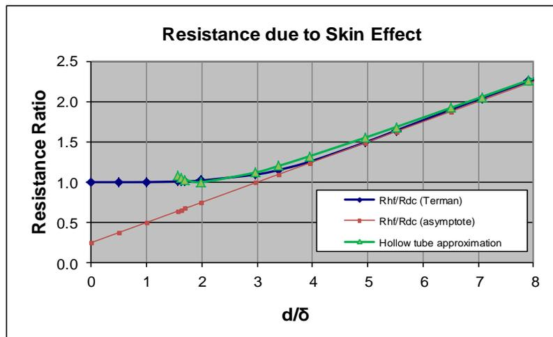
Figure 2.3.2 Resistance of Round Wire at High frequencies
