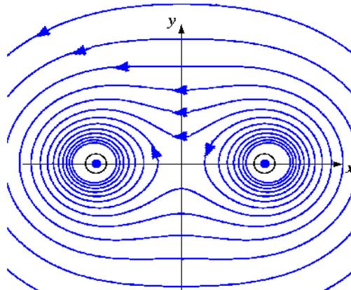
Figure 3.1.1 Lines of constant  $H$  around Two parallel Wires carrying Similar Currents
