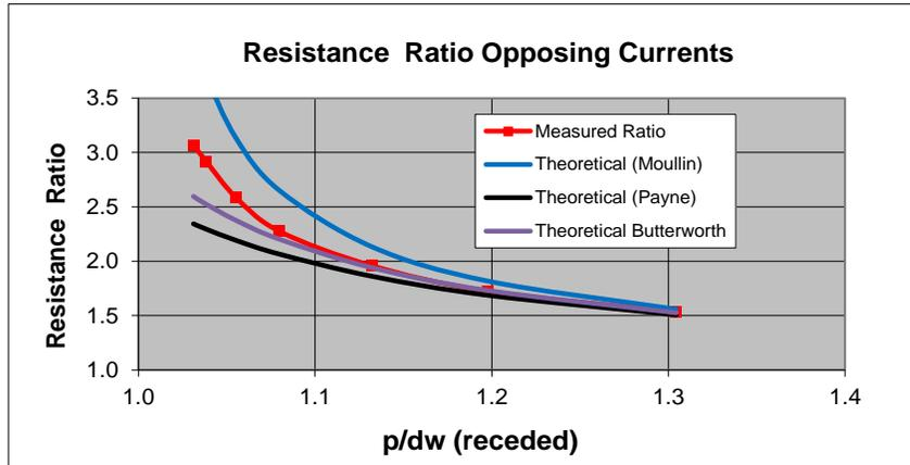
Figure A3.3.1 Resistance Ratio for Opposing Currents, Measured and Theoretical
