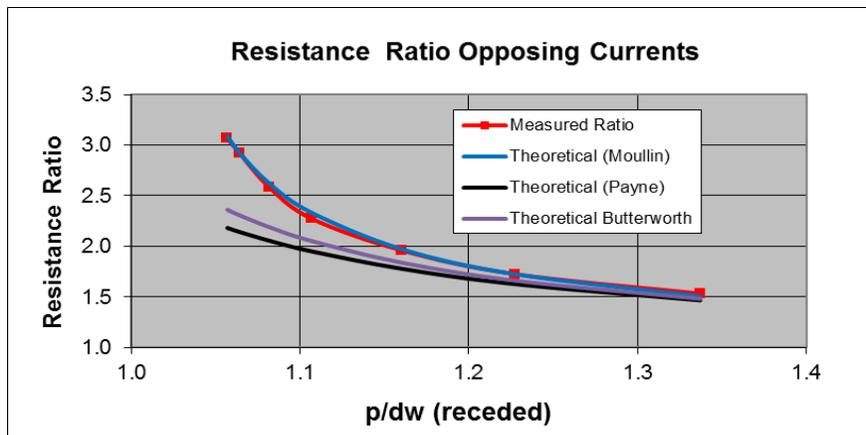
Figure A3.3.2 Resistance Ratio for Opposing Currents, Measured and Theoretical
