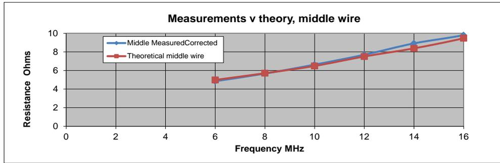
Figure 5.4.1 Resistance of Middle Wire of Five Wires
