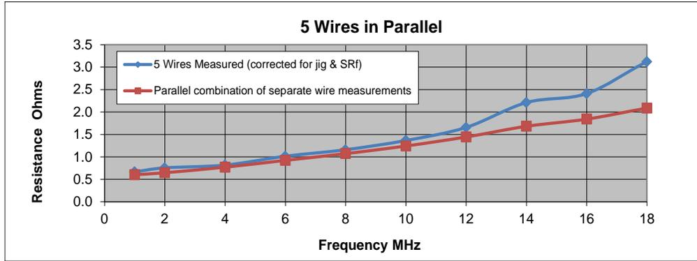
Figure A5.3.1 Resistance of Wires in a Group of Five
