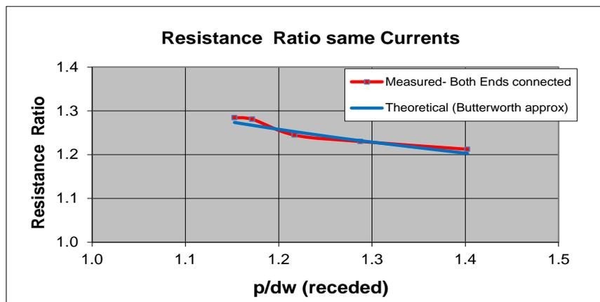
Figure 3.3.2.1 Resistance Ratio for Currents in Same Direction
