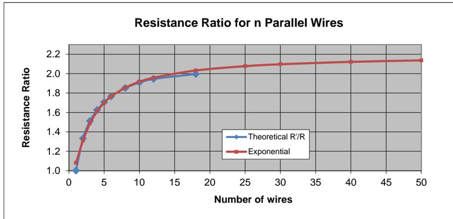
Figure 5.4.1 Resistance Ratio for n Parallel Cylindrical Wires
