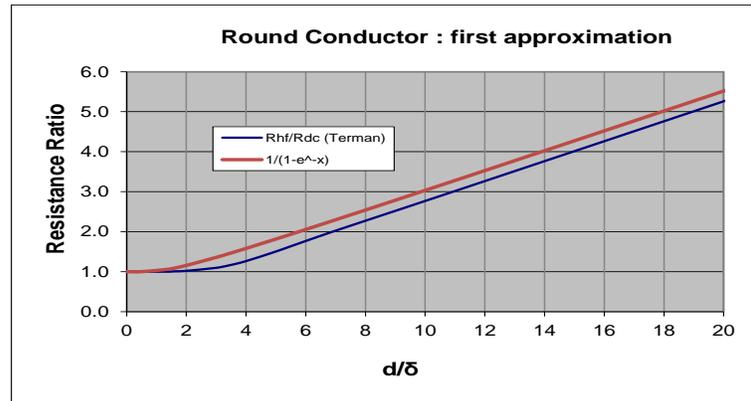
Figure A6.1 Round Conductor : first approximation
