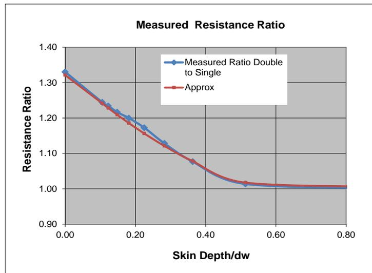
Figure 3.3.5.2 Empirical equation for proximity loss
