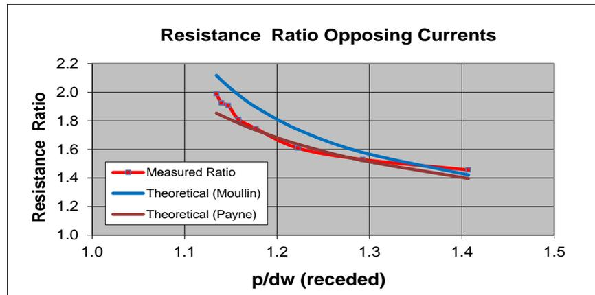
Figure A 3.2.1 Resistance Ratio for Opposing Currents, Measured and Theoretical
