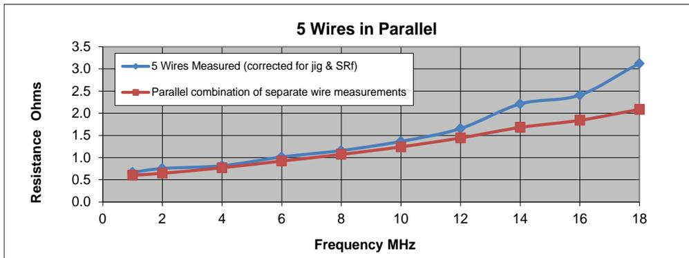
Figure 5.3.1 Resistance of 5 Wires side by side
