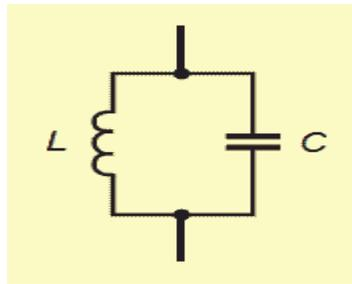
Figure 5.1 Equivalent circuit for self-resonance
