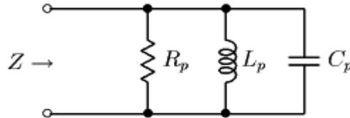
Figure 8.1.2 Self-capacitance model with Loss
