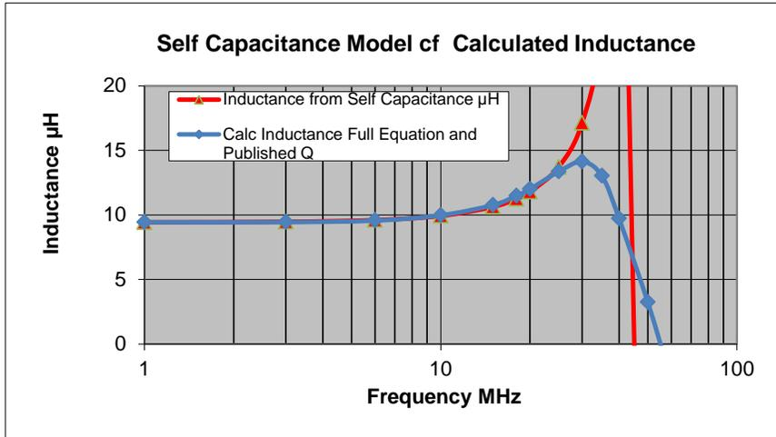
Figure 7.2.1 Self Capacitance Model and Measured Inductance Matl 61
