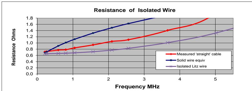
Figure 6.6.1 Resistance of 'Straight' Cable
