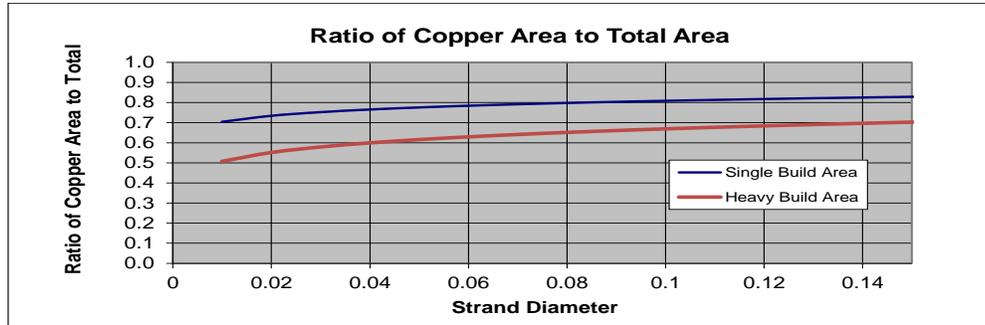
Figure 2.3.2 Ratio of Strand copper area to area with insulation
