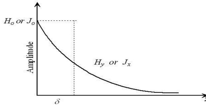
Figure 10.1.1 Current density at high frequencies
