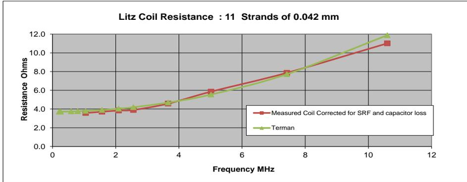
Figure 6.5.2 Resistance of coil
