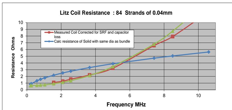
Figure 6.6.2 Comparison of Theory and Measurements
