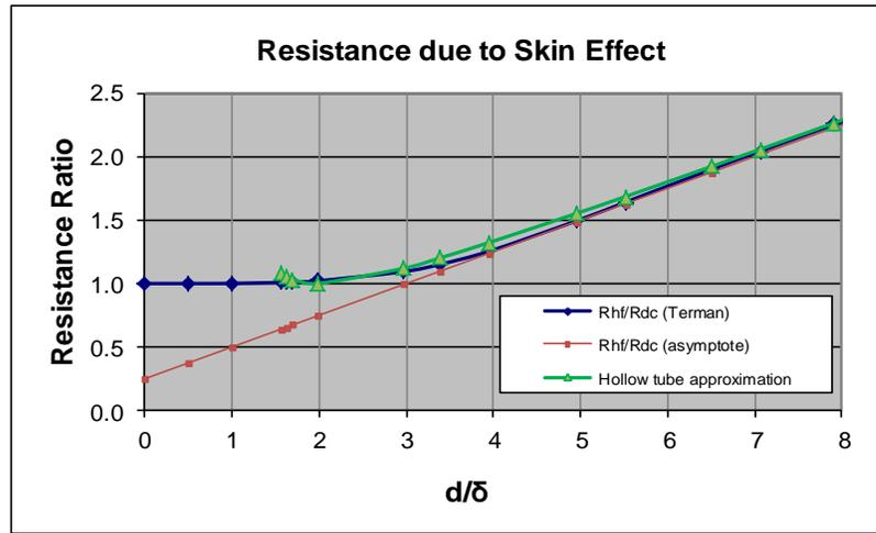
Figure 10.2.2 Resistance at high frequencies
