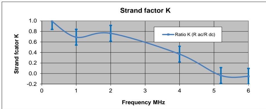
Figure 9.1 Effect of broken Strands
