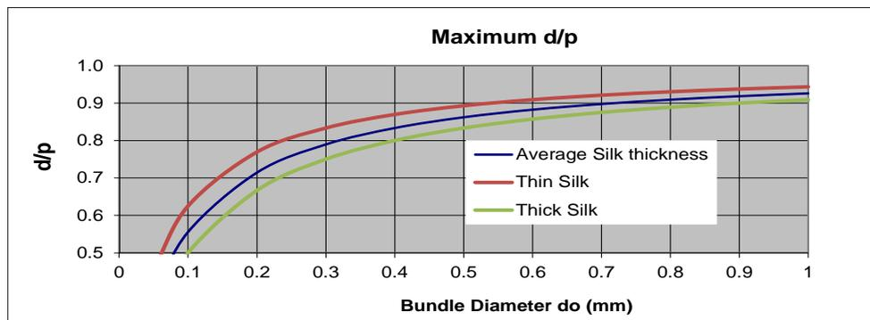
Figure 2.4.1 Maximum  $d_o/p$  due to Silk Insulation
