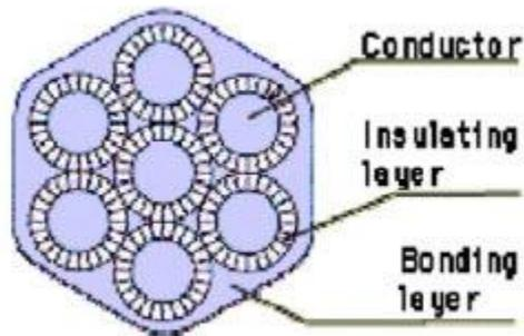
Figure 2.1 Cable with 7 Insulated Strands
